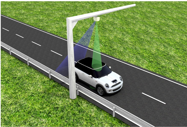
Detection beams radar (blue) and ultrasound (green)
